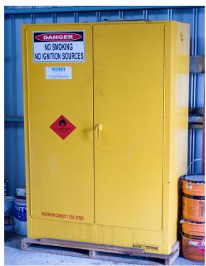
Depending on the volumes stored products should be held in purpose-built cabinets/buildings, stored on bunded pallets / trays or in a bunded area that is isolated from stormwater runoff.
